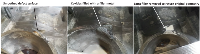
Fig. 1 The three main phases of refurbishing metal dies. (Original photos Matteo Perini)
